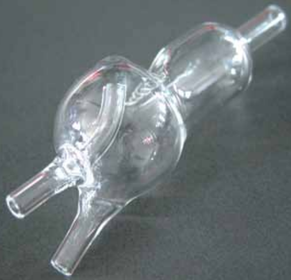
▲ Gas and Liquid Separator
